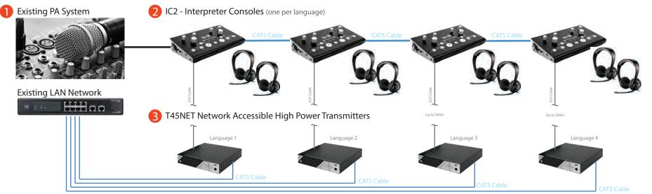
\*Transmitters to be placed closest to audience area for best transmission coverage \* ANT005 antennas can use WCA008 15m coaxial extension cables for longer reach.
